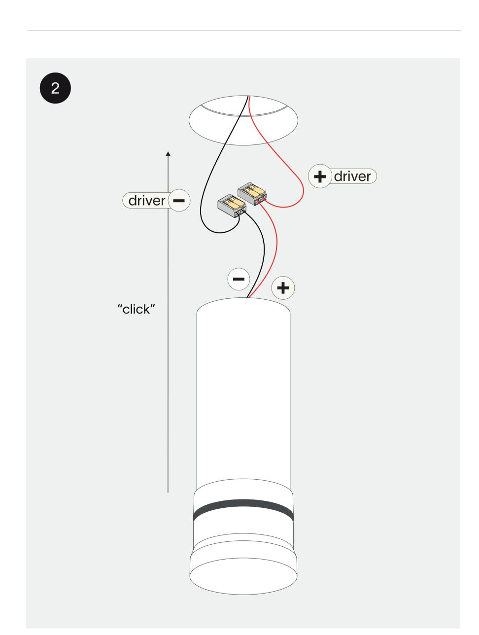
Connect the wires with wago connectors.
