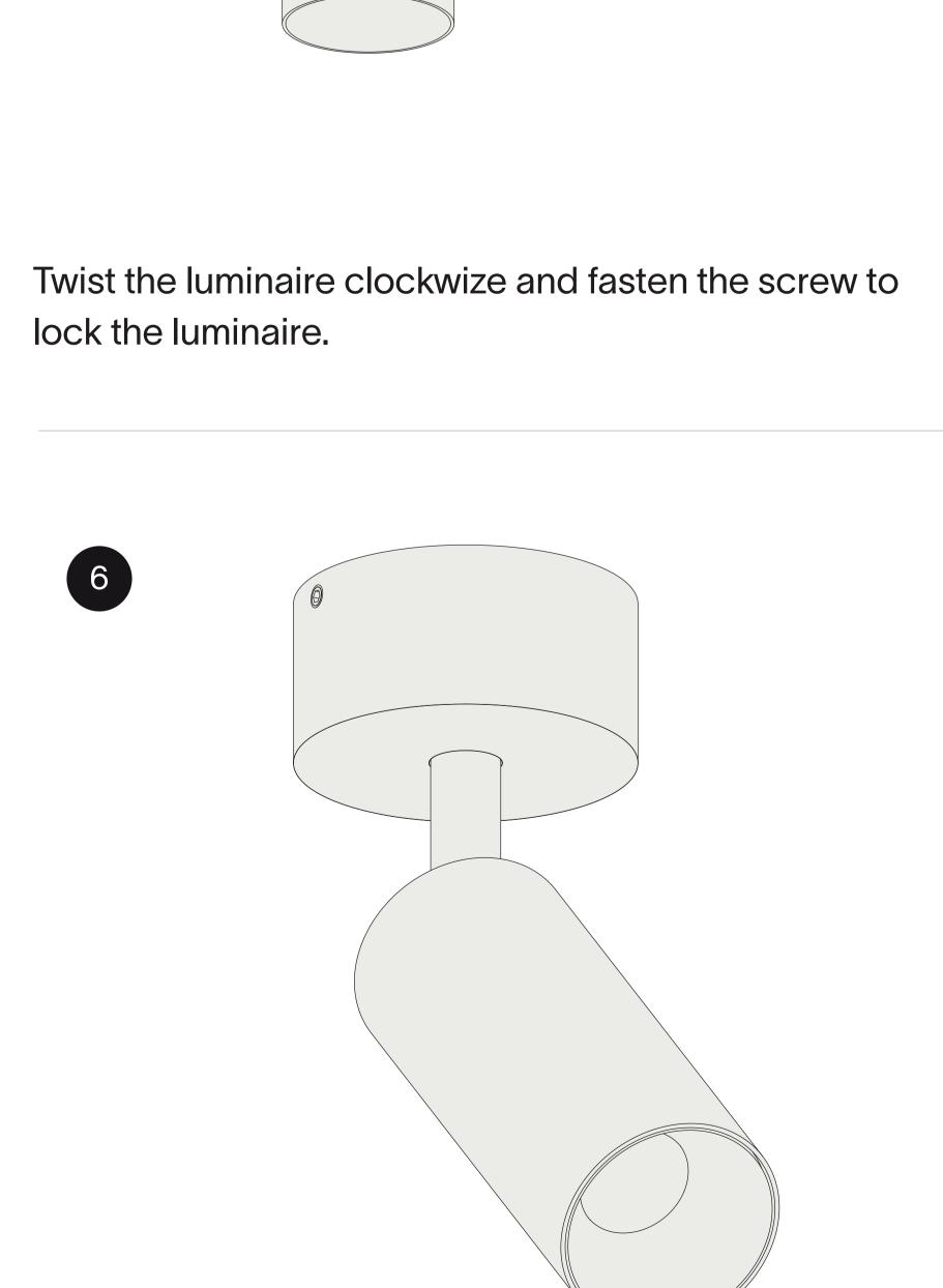
Tilt the luminaire as desired and turn the power back on.
