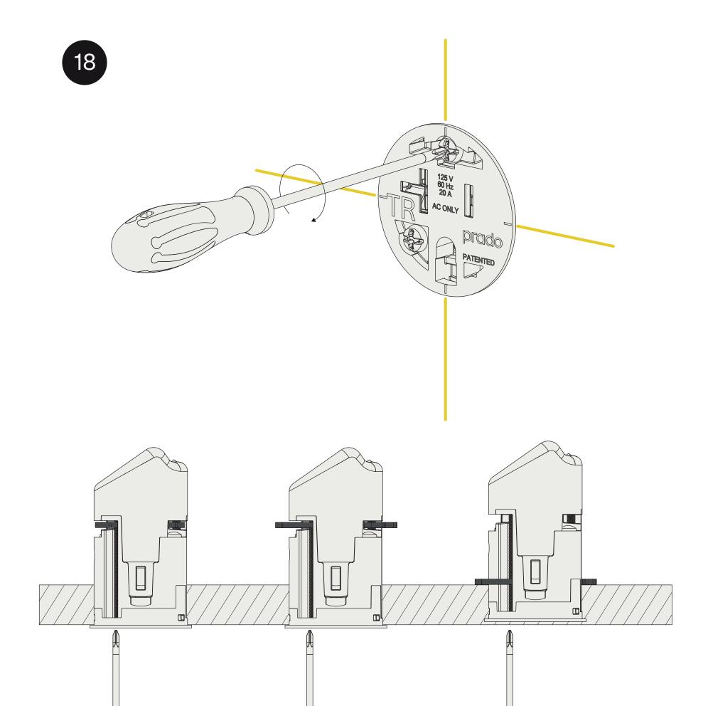
Level the outlet and fixate it by tightening the screws.
