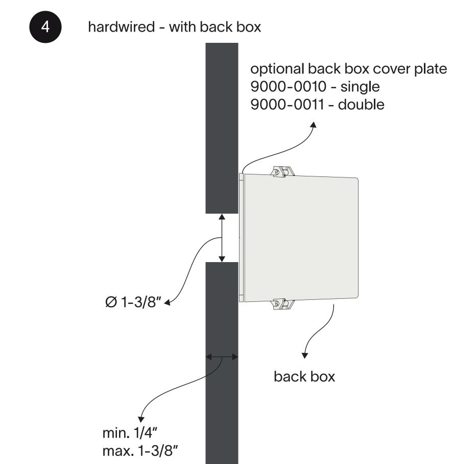
Drill the installation hole and optional countersink.
