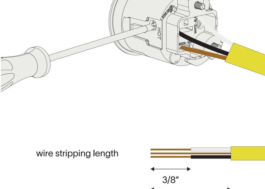
Make all necessary connections, make sure correct
