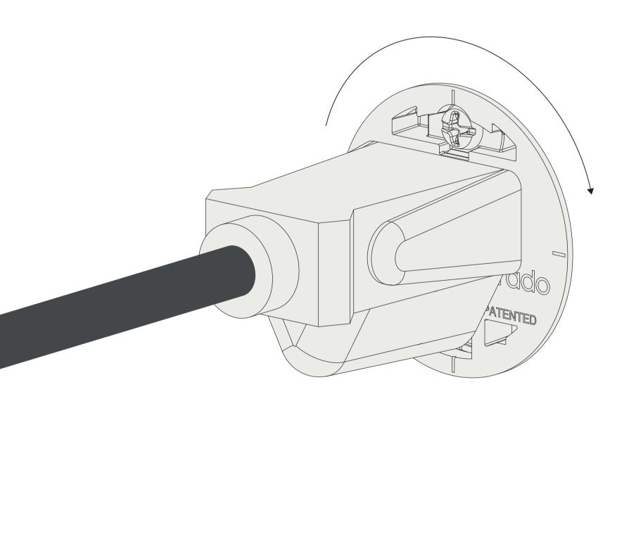
Remove the outlet by using a plug and twisting clockwise.
