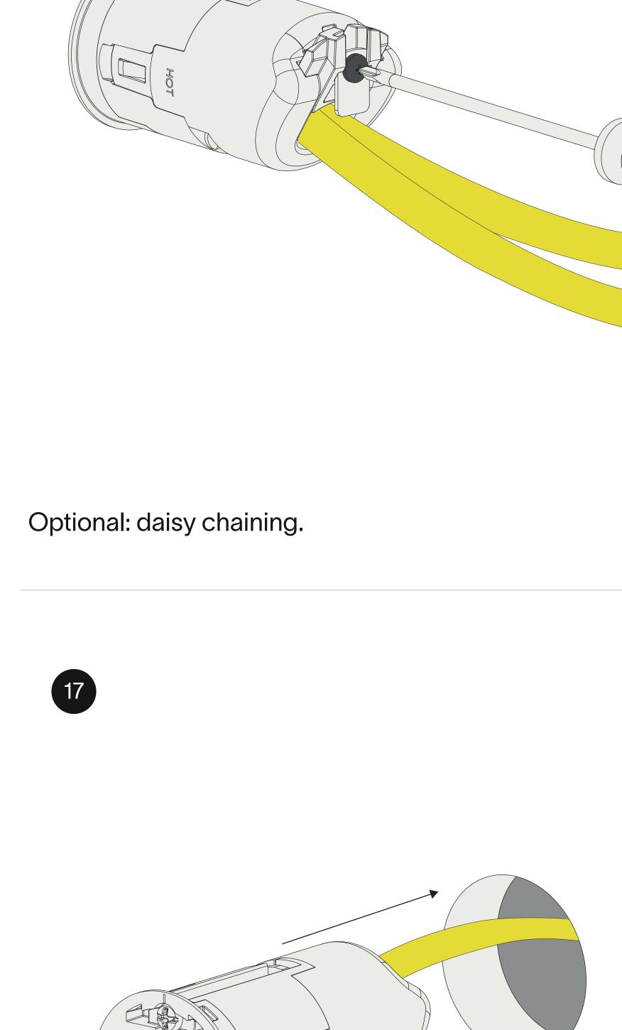
Insert the outlet in the hole and go to step 18 (click here)
