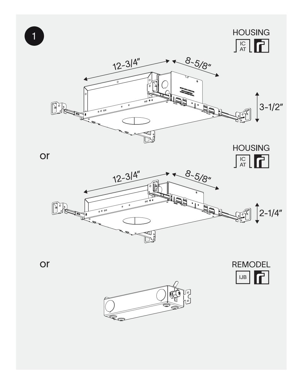
Install the appropriate IC recessed box/driver box.
