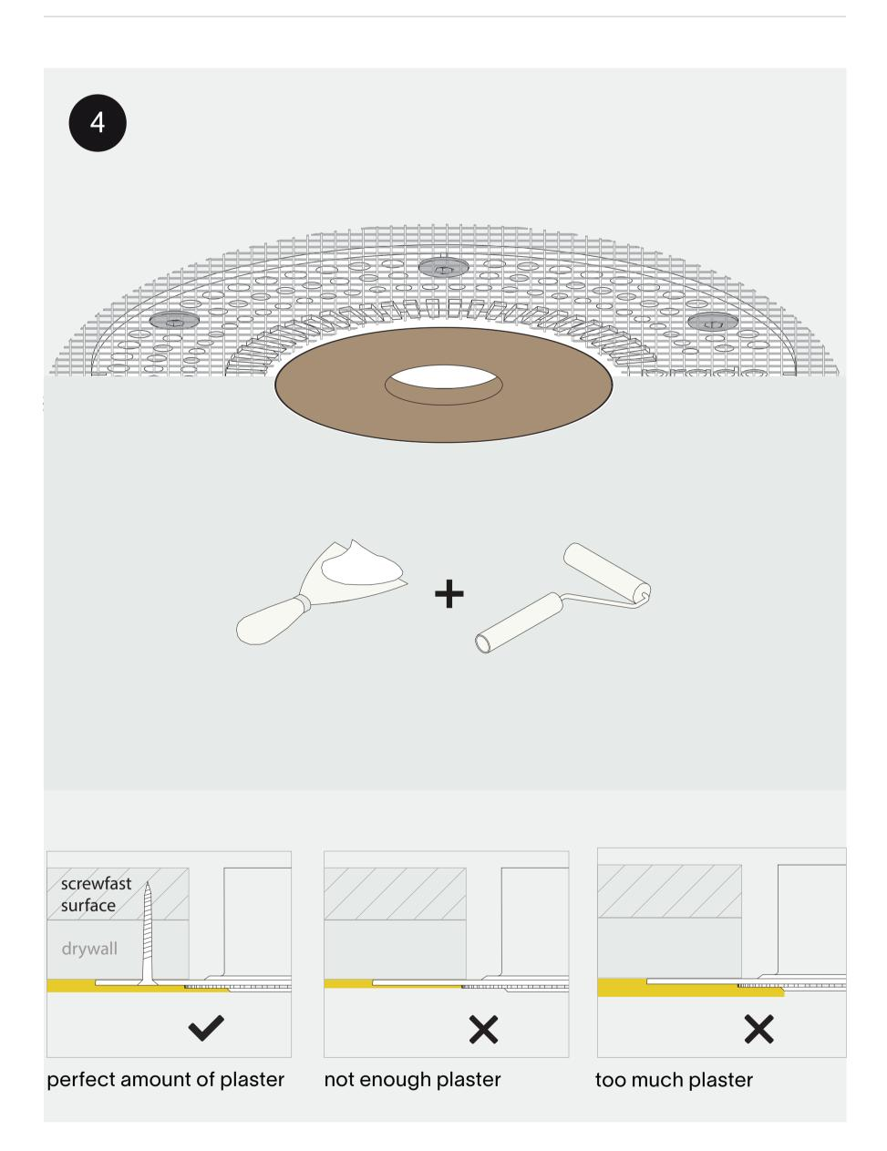
Excercise caution while plastering, do not damage the ring. Keep the plaster lid inside the mud ring while plastering. Use a fiberglass mesh tape for optimal plaster adhesion. Make sure not to touch the edge of the ring when sanding.
