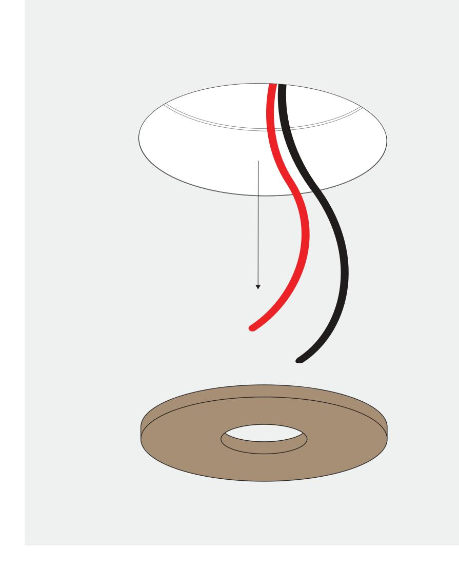
Remove the plaster lid before installing the fixture. Any residue needs to be removed without damaging the edges of the ring.
