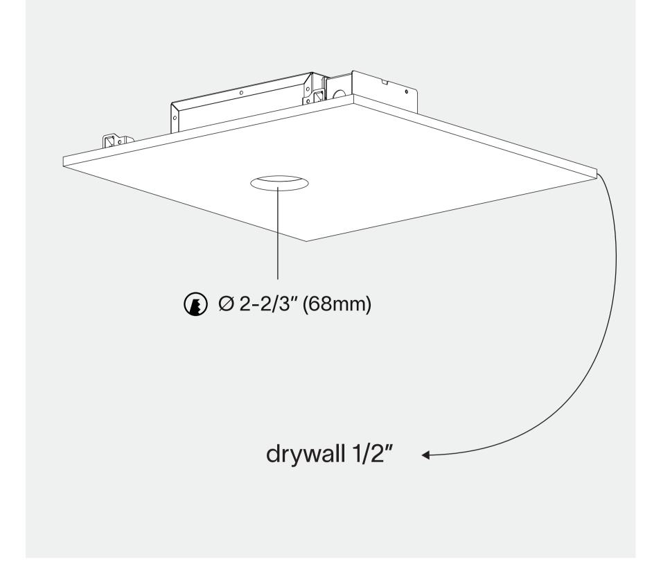
Install the drywall (thickness 1/2'') with a round hole (Ø 2-2/3'').
