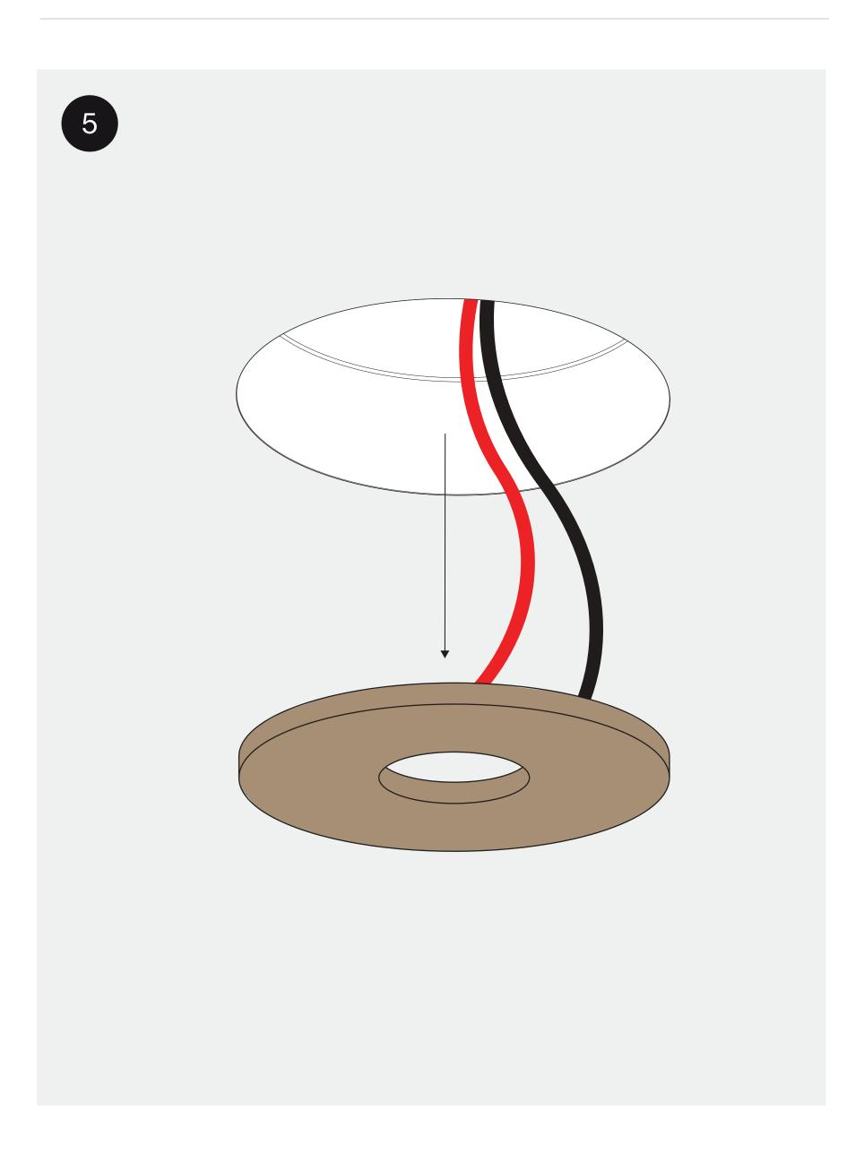
Remove the plaster lid before installing the fixture. Any residue needs to be removed without damaging the edges of the ring.
