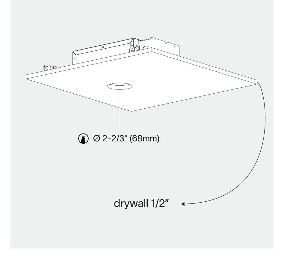
Install the drywall (thickness 1/2'') with a round hole (Ø 2-2/3'').
