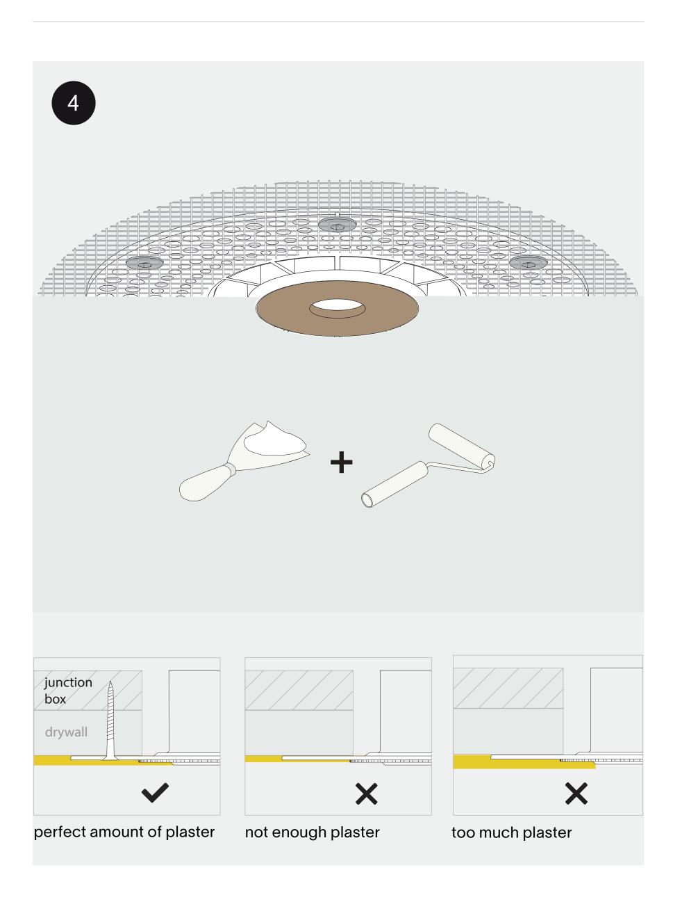
Excercise caution while plastering, do not damage the ring. Keep the plaster lid inside the mud ring while plaster tering. Use a fiberglass mesh tape for optimal plaster
