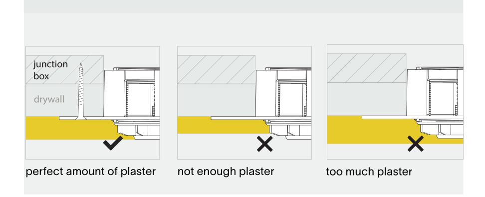
Excercise caution while plastering, do not damage the ring. Keep the plaster lid inside the mud ring while plastering. Use a fiberglass mesh tape for optimal plaster adhesion. Make sure not to touch the edge of the ring when sanding.
