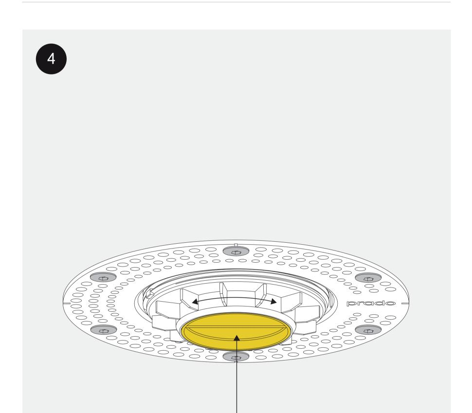
Adjust the height of the mud ring by twisting the inner part of the kit (min. 9/64" (3.6mm) - max. 3/4" (20mm)).
