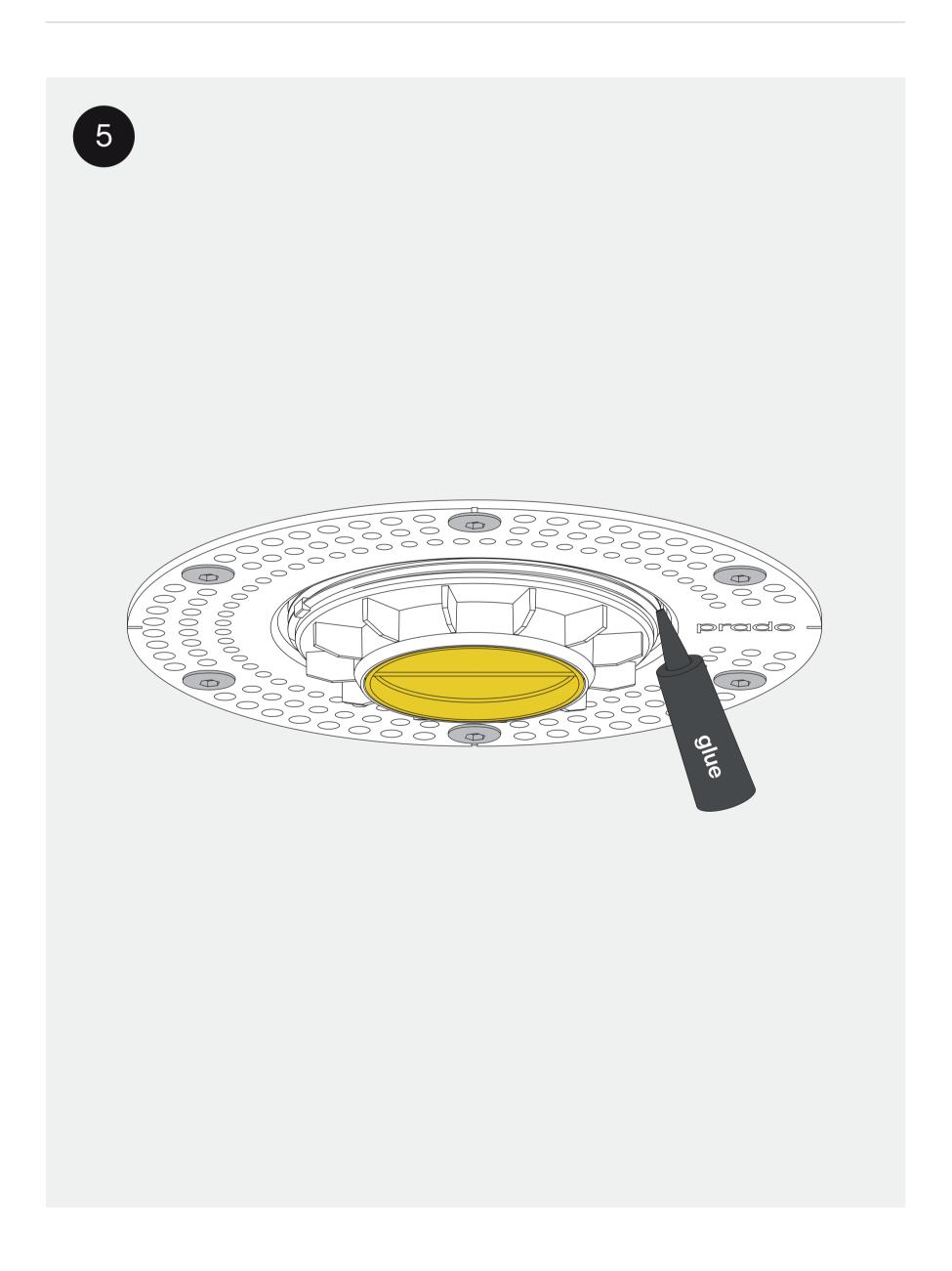
Fixate the inner part with the appropiate glue.
