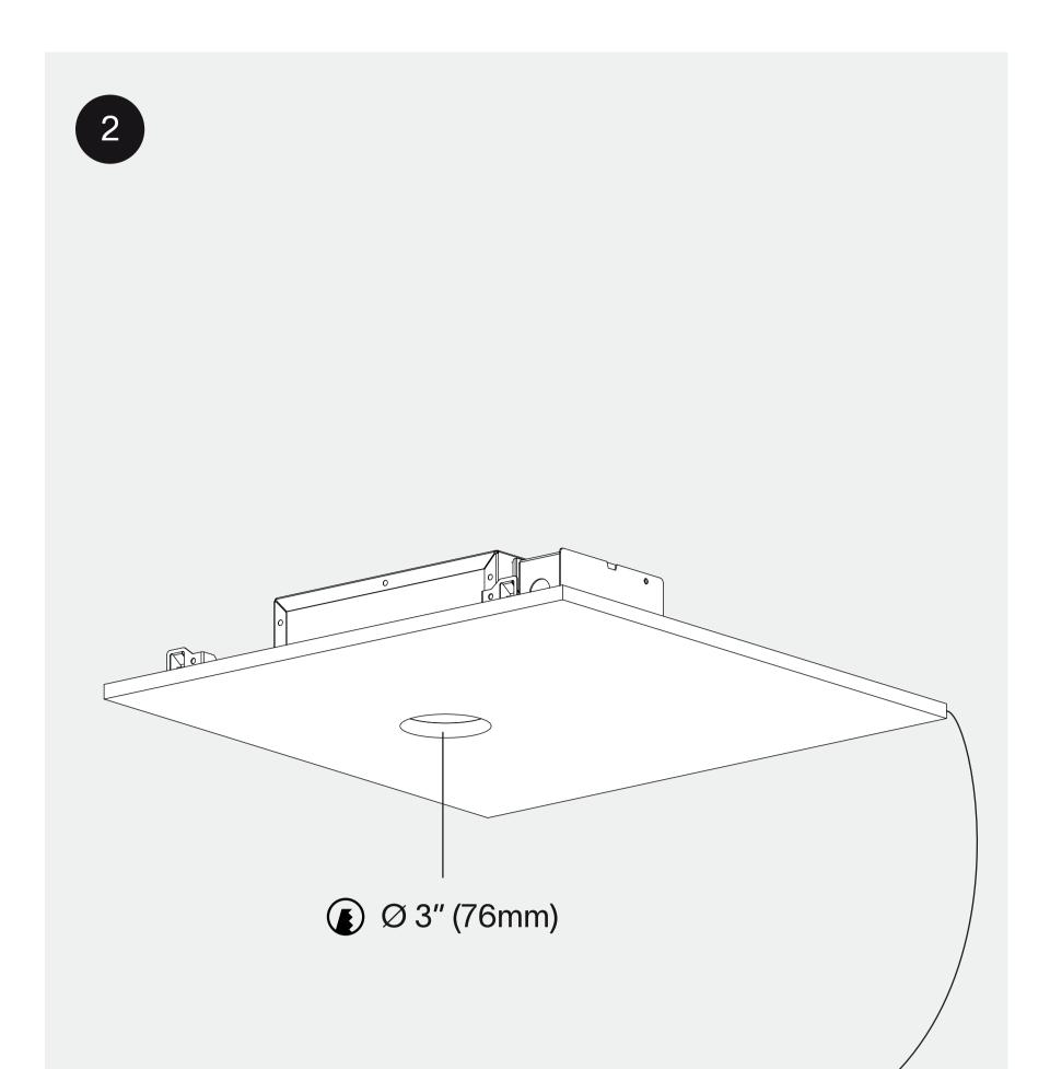
Install the drywall (thickness 1/2'') with a round hole (Ø 3'').
