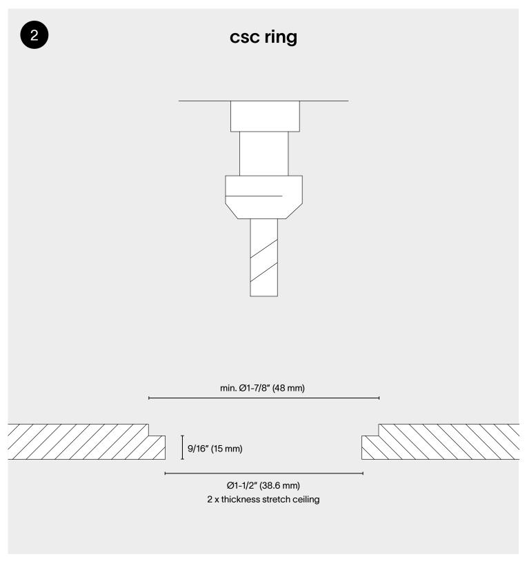
Mill a round hole with the above dimensions in a wooden base (not supplied) (max. fabric thickness: 3/64" (1.2 mm)).
