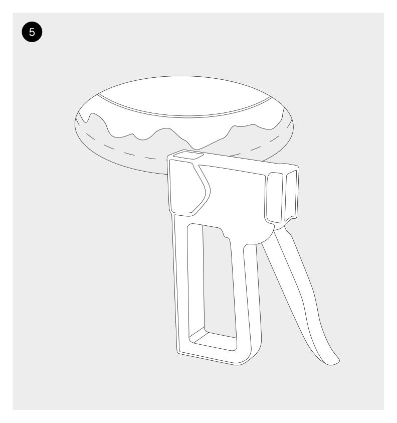
Fasten the cloth in the wooden base (below the csc kit). Cut off the excess fabric (it cannot touch the csc ring).
