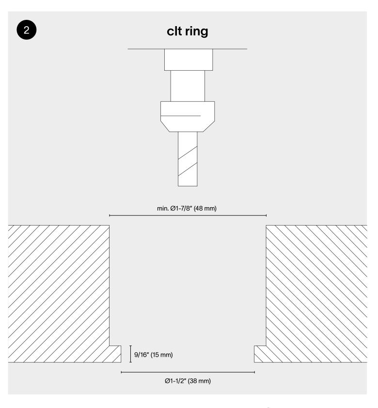
Mill a round hole with the above dimensions. Consult the chosen luminaire tech specs for required height and free air dimensions.
