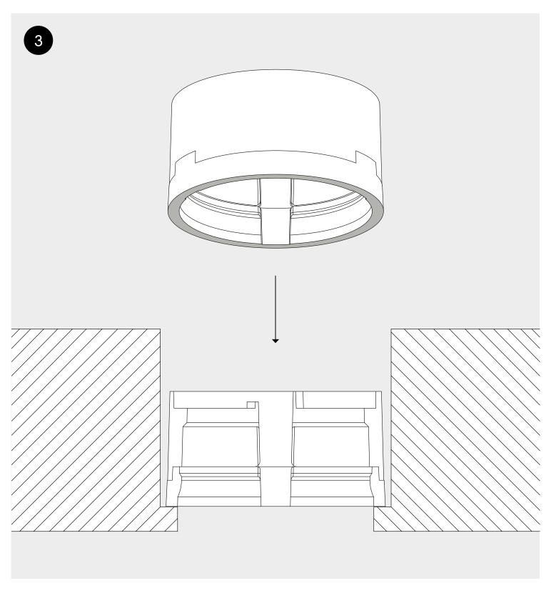
Place the clt ring in the hole, grey side facing down.
