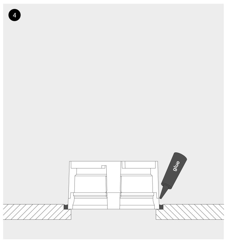
Fixate the csc ring to the wooden base with the appropriate glue.
