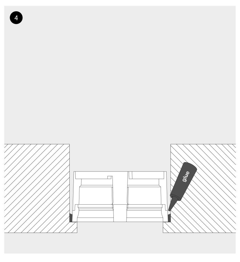
Fixate the ring to the clt with the appropriate glue.
