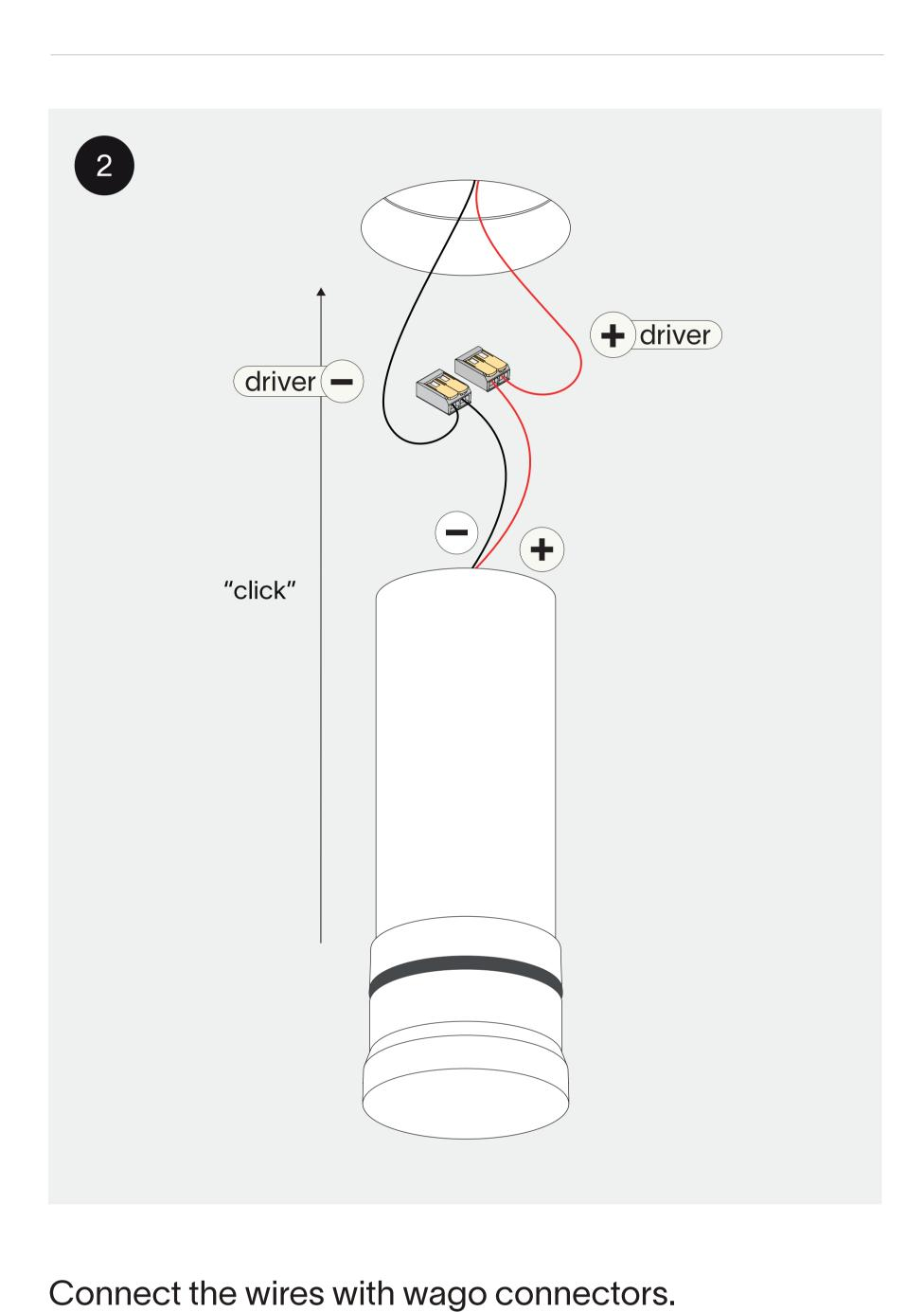
For serial connection, respect polarity.
