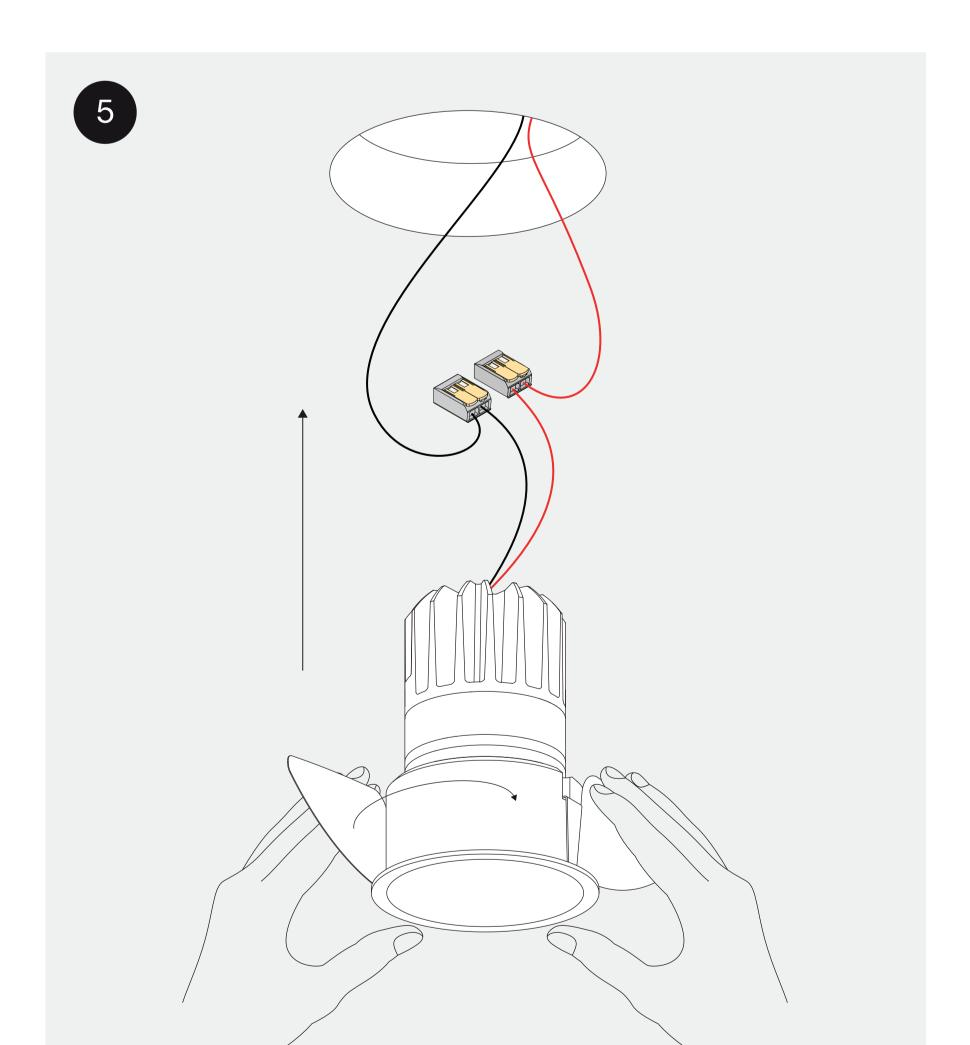
Bend over the springs and push the luminaire into the ceiling.
