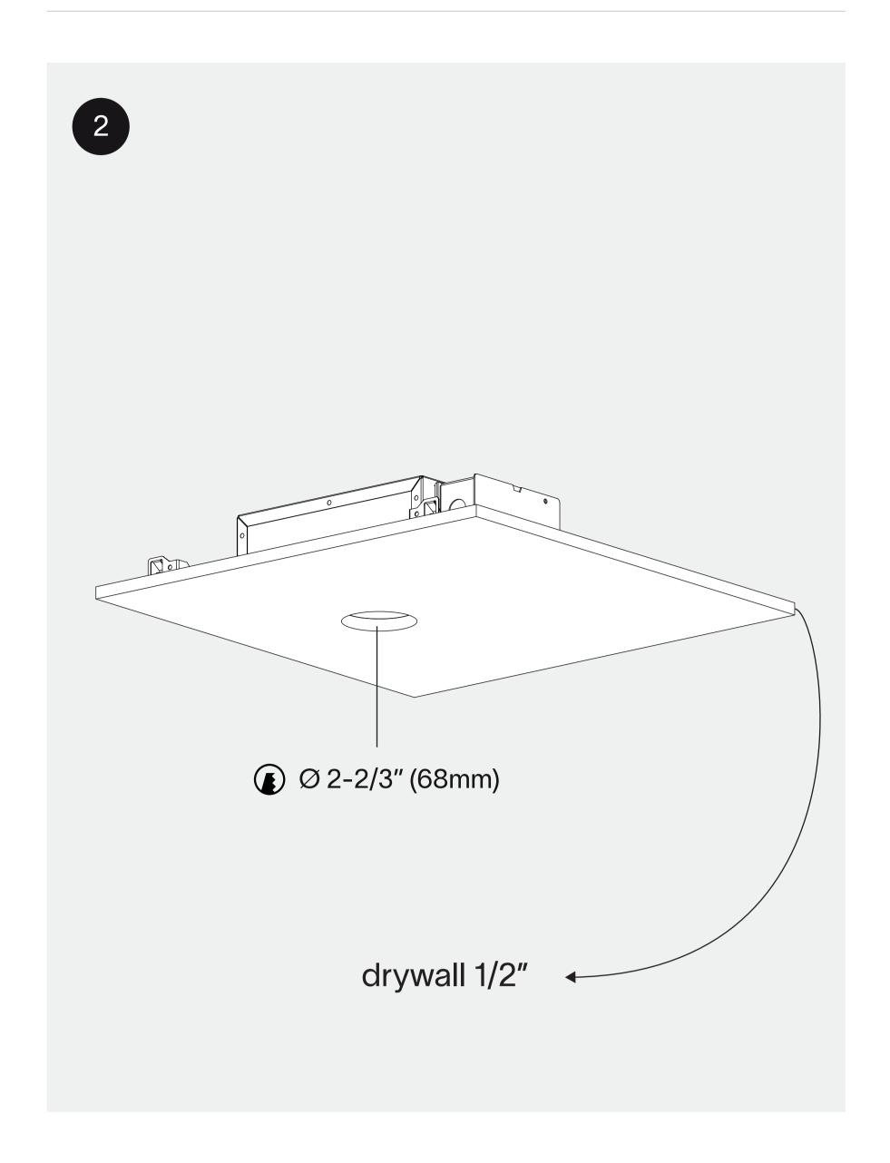
Install the drywall (thickness 1/2'') with a round hole (Ø 2-2/3'').
