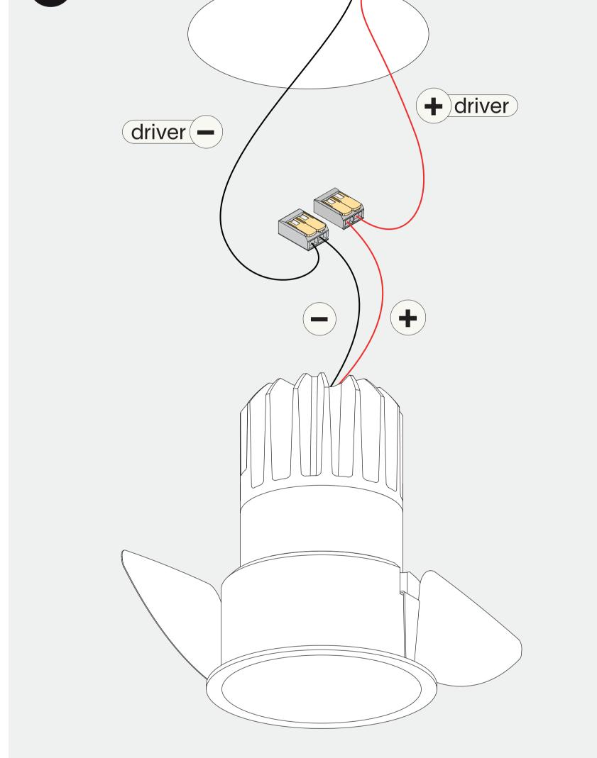
Connect the wires with wago connectors. For serial connection, respect polarity. Combine with a prado LED-driver.
