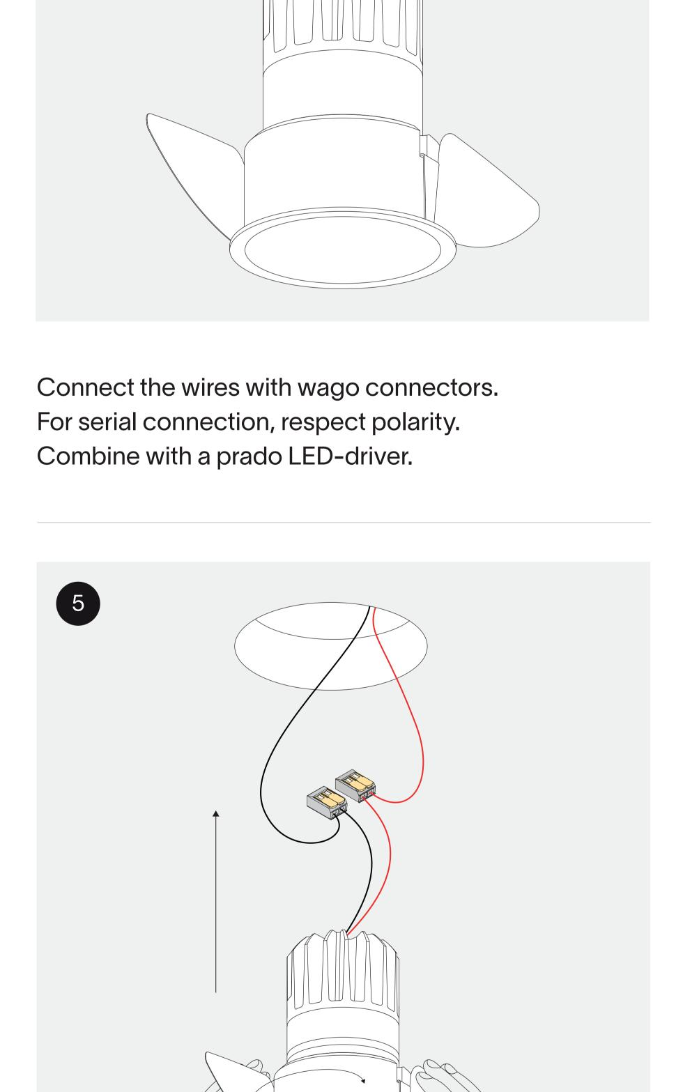
Bend over the springs and push the luminaire into the
