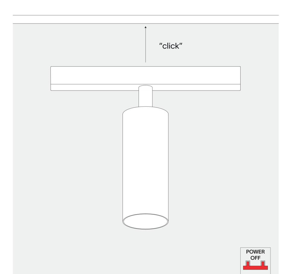
slide the luminaire in the prado 48V track make sure to use a prado 48V LED-driver
