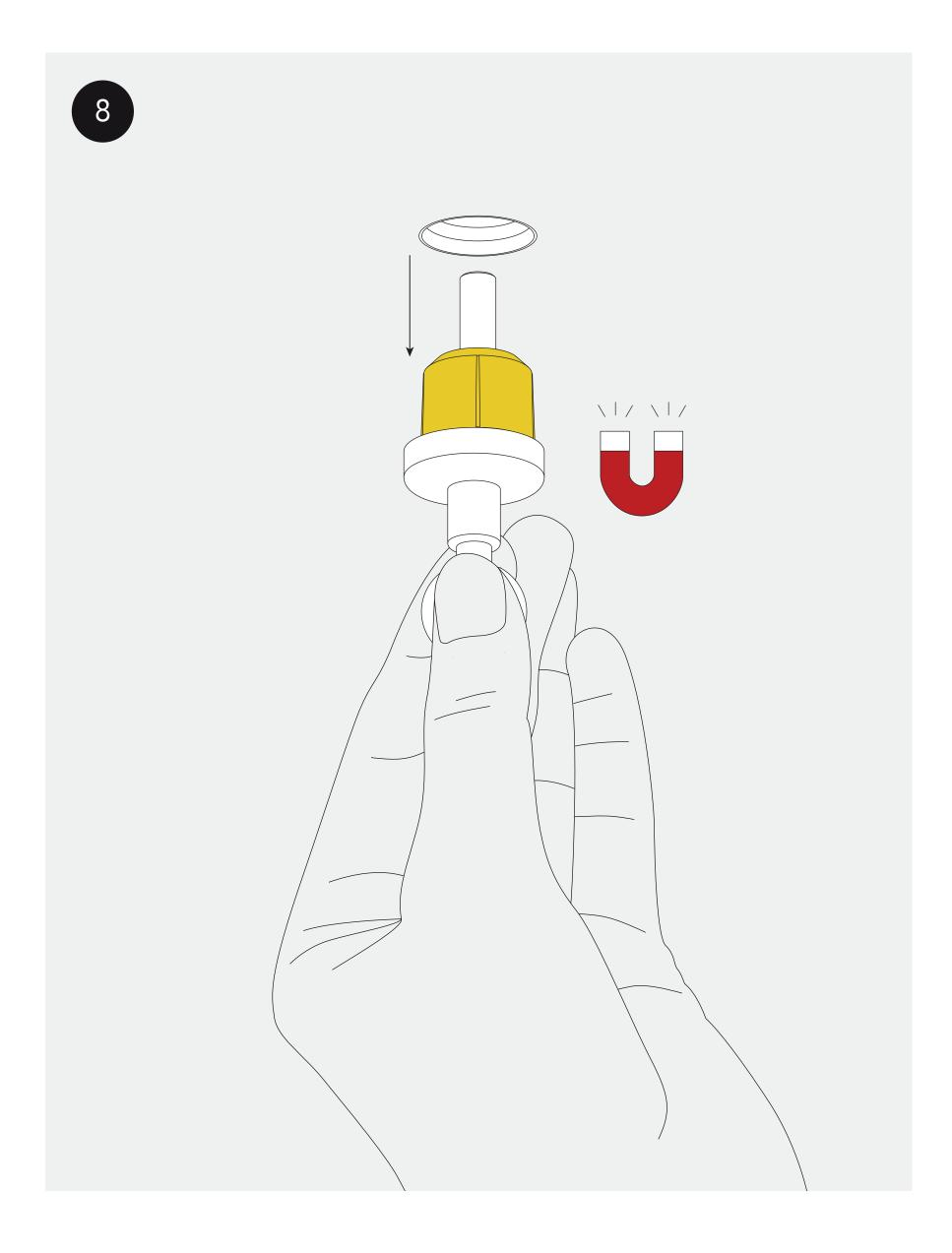
Remove the plaster lid with a magnet before installing the fixture. Any residue needs to be removed without damaging the edges of the installation ring. Thank you for choosing prado.
