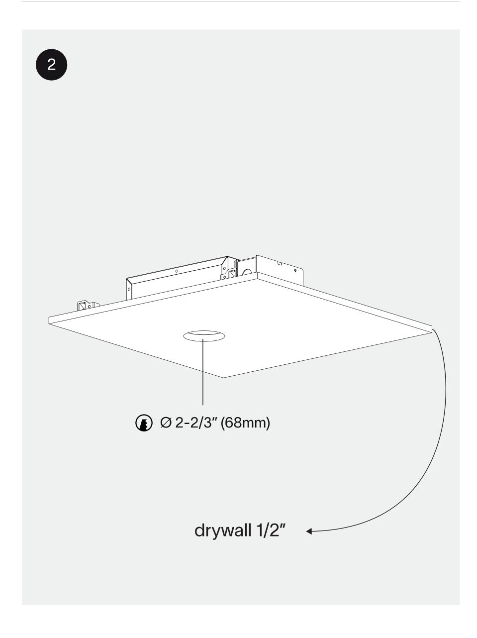
Install the drywall (thickness 1/2") with a round hole (Ø 2-2/3").
