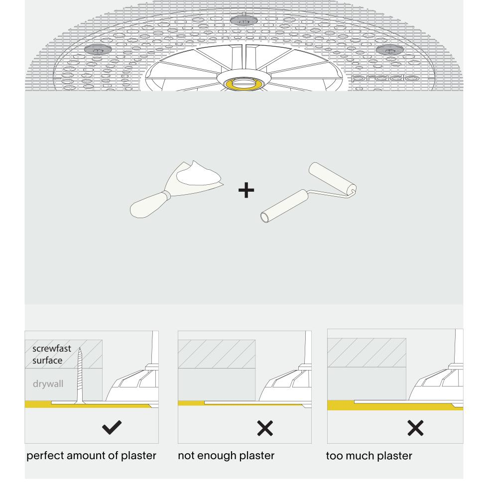
Excercise caution while plastering, do not damage the ring. Keep the plaster lid inside the mud ring while plastering. Use a fiberglass mesh tape for optimal plaster adhesion. Make sure not to touch the edge of the ring when sanding.
