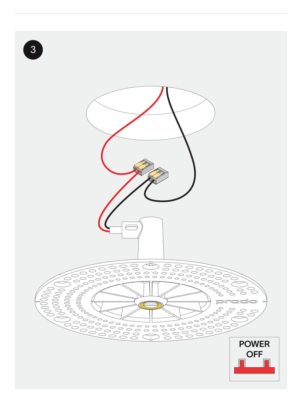
Connect the wires with wago connectors. For serial connection, respect polarity.
