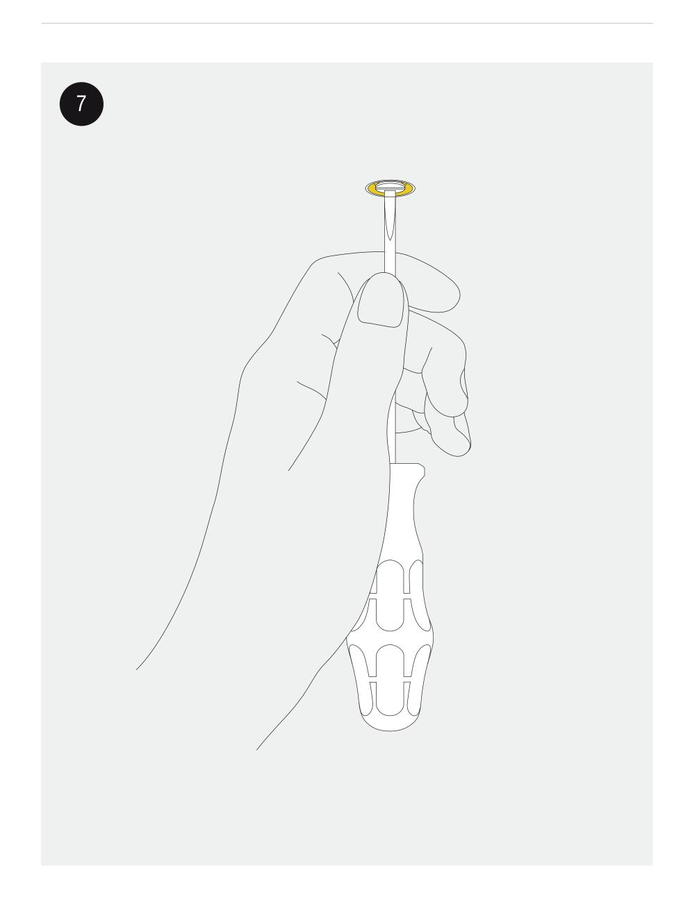
Twist the yellow plaster lid with a screwdriver before removing it with a magnet.
