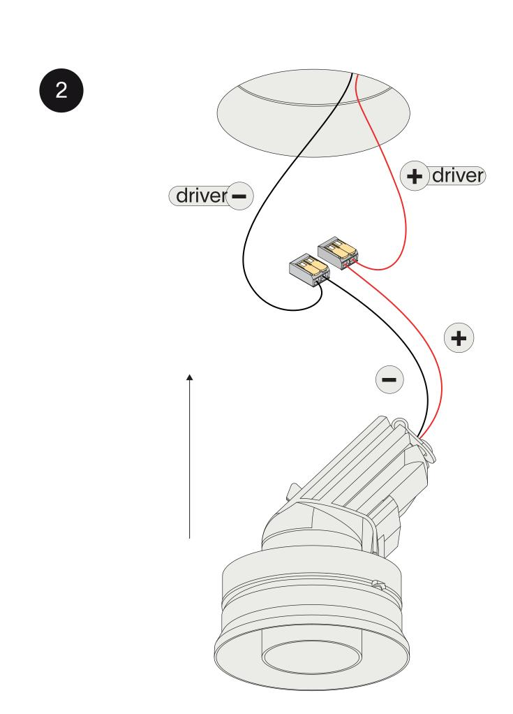
For serial connections, respect polarity. Combine with a prado LED-driver.
