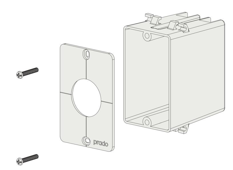
Install the cover plate onto the back box.
