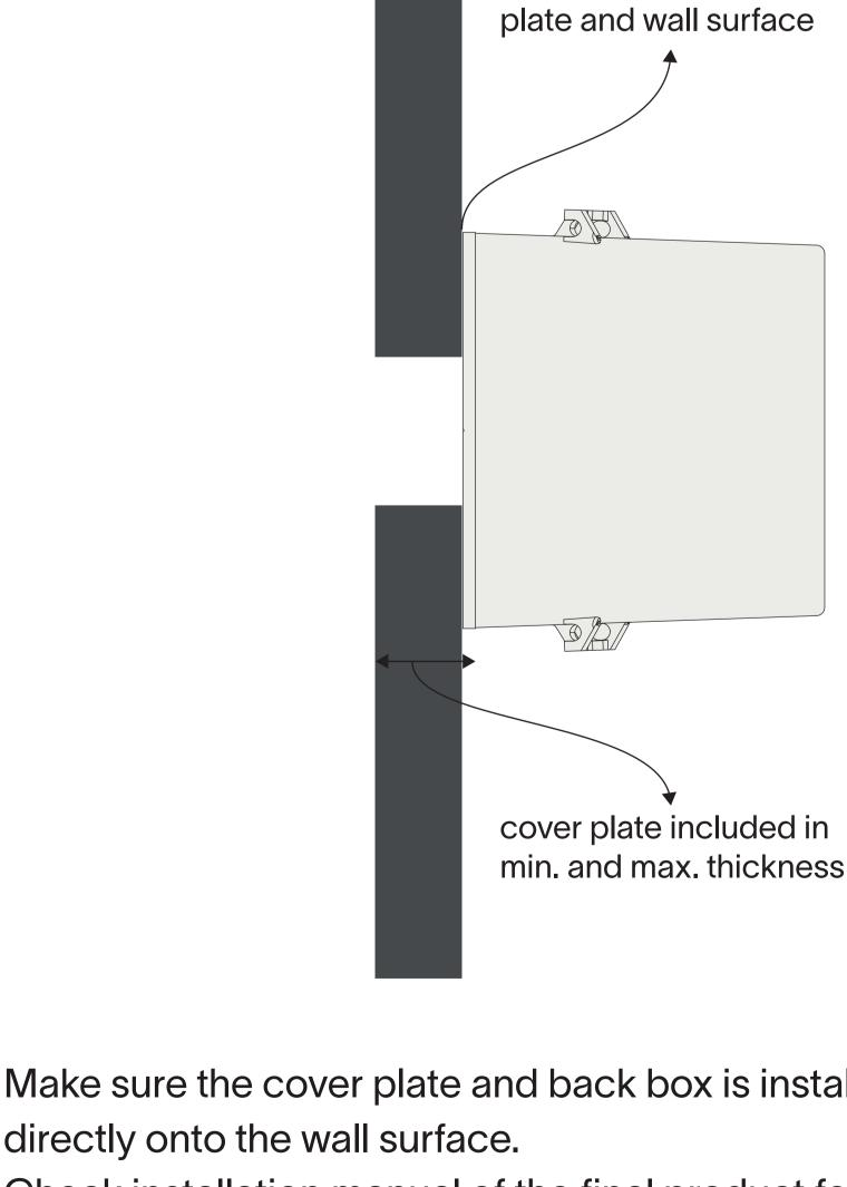
Make sure the cover plate and back box is installed
