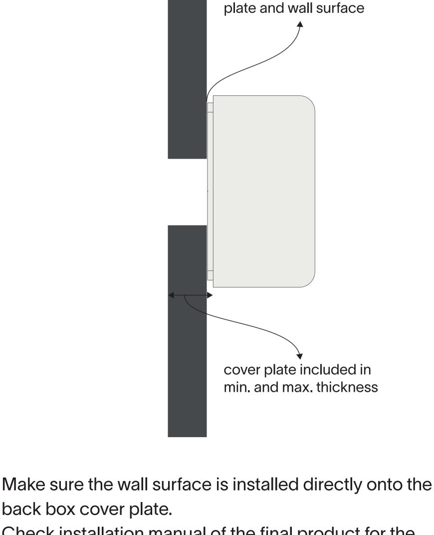
Check installation manual of the final product for the minimum and maximum thickness of the wall surface. Make sure to include the back box cover plate into this thickness.
