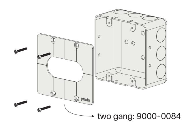
Install the cover plate onto the back box. Both metallic and plaster back boxes are possible.
