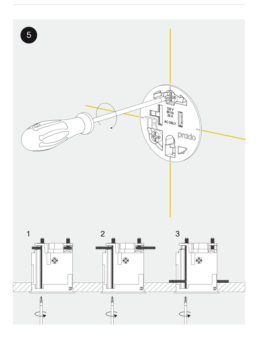
level the outlet and fixate it by tightening the screws
