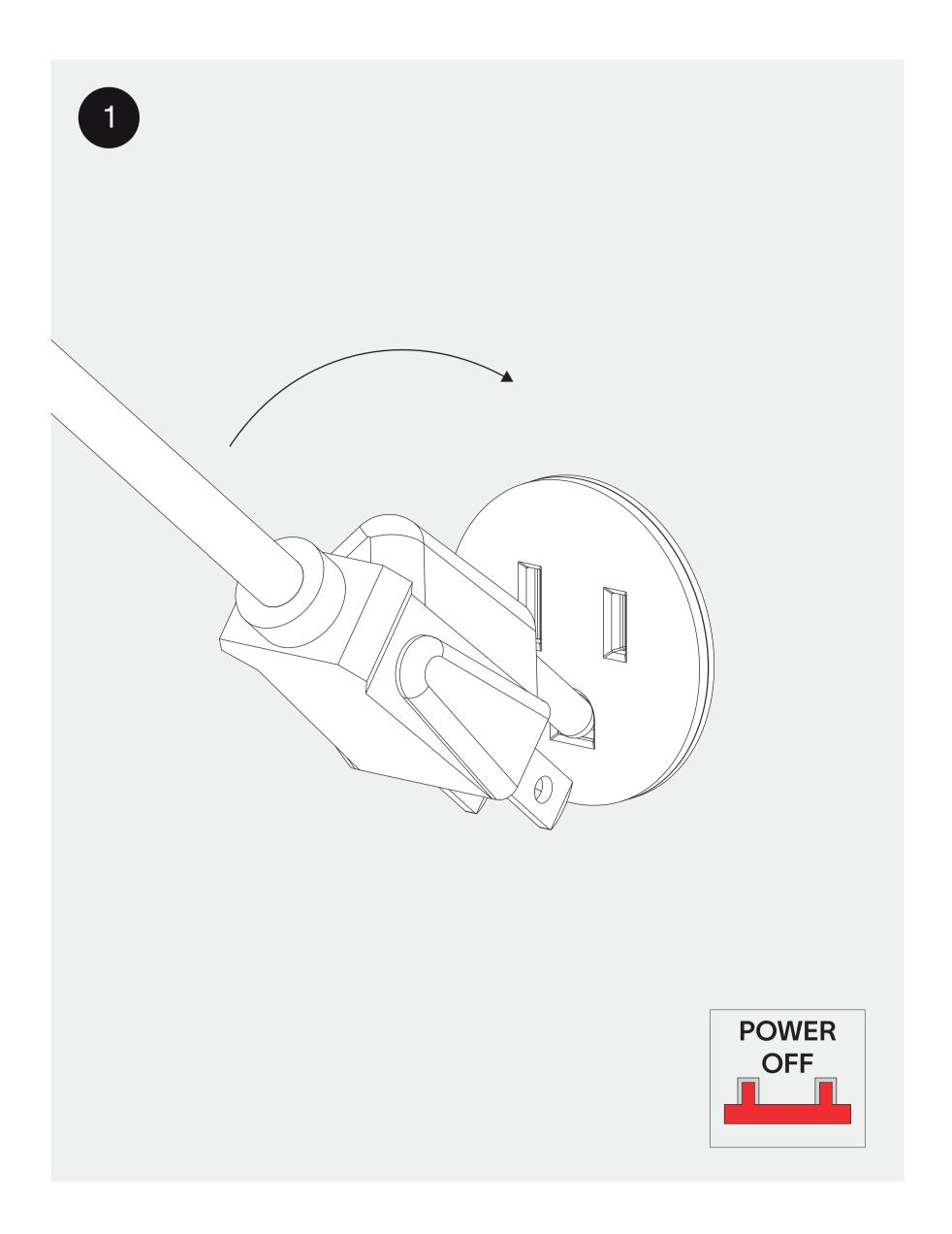
turn the power off before removing the outlet
