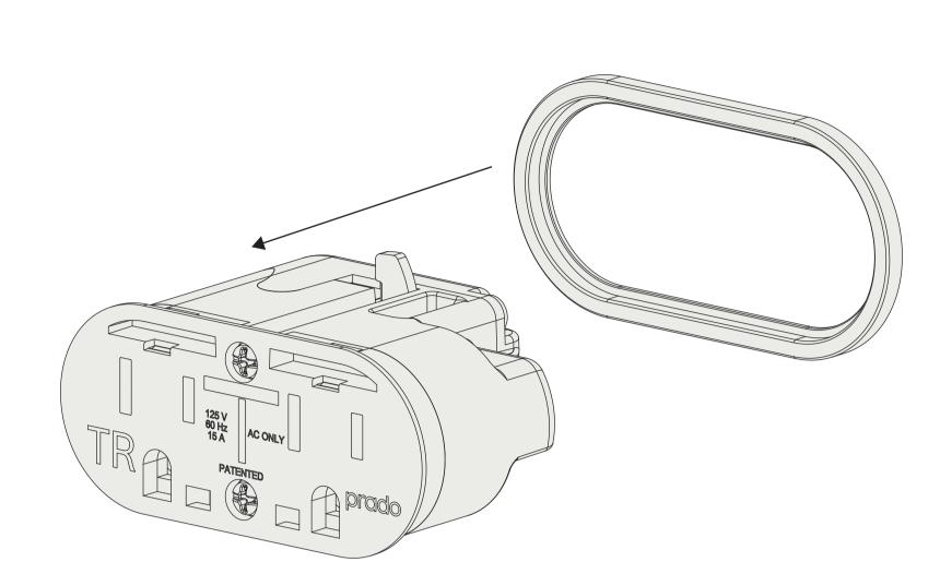
Slide the small trim ring over the outlet before installing the outlet.
